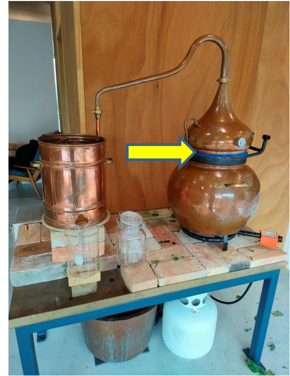
Hydro-distillation 8kg Piper Excelsum 21 Litres water Targeting Hydrosol
